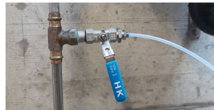
Figure 5: Simple control of the required water flow rate of 200 to 400 ml/min when continuously measuring with the BactoSense
