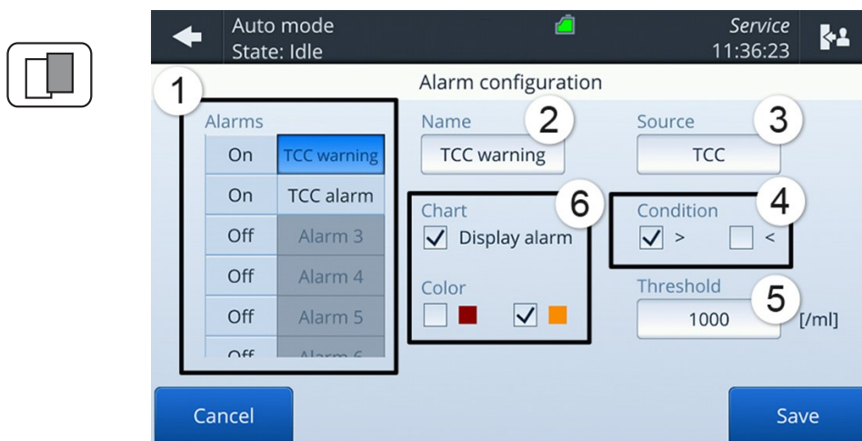
Figure 2-1 Alarm configuration in the BactoSense graphical user interface.
