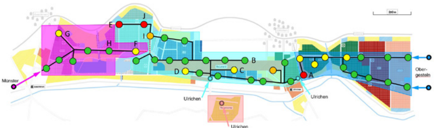
Figure 1: The temporary network with the four subnetworks Münster (violet), Ulrichen (turquoise, pink) and Obergesteln (blue). At point H, BactoSense was permanently installed and provided continuous measurement data. Manual grab samples for BactoSense were taken randomly or when there was a concern. The advantage of BactoSense over classical plating methods is that results are achievable within 20 mins. At point J, a contamination event occurred, which will be discussed in section „Complementarity between rapid detection and lab analysis“.
