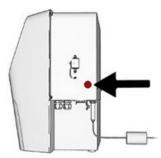
2. Power on the autosampler. The green lamp on the front panel of the autosampler will turn on.
