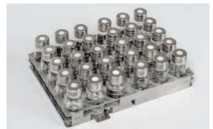
Sample tray containing up to 30 vials
