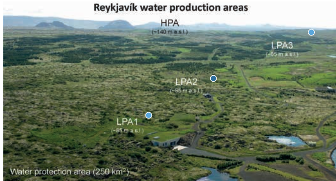
Figure 1: Veitur Water Utilities extracts from several boreholes spread across protected areas situated either in low areas LPA (85 m a.s.l.) or in high areas HPA (140 m a.s.l.). Each area has its own maximum capacity. The blue dots indicate the positions where BactoSense is installed.
